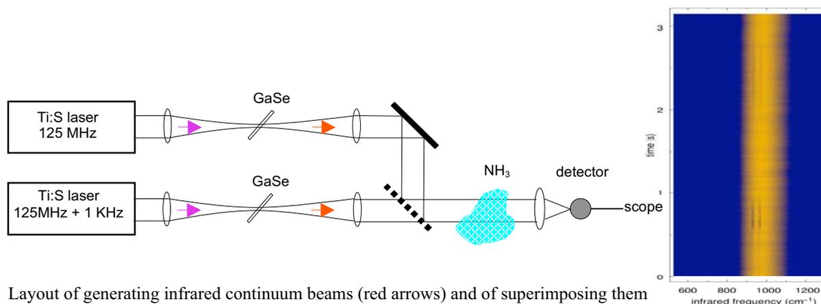
Layout of generating infrared continuum beams (red arrows) and of superimposing them to obtain self-scanned interferograms on an HgCdTe detector. Right panel: approx. 3000 spectra taken in 3s of continuous recording testify to a time-varying  $\text{NH}_3$  mass in the beam path.
