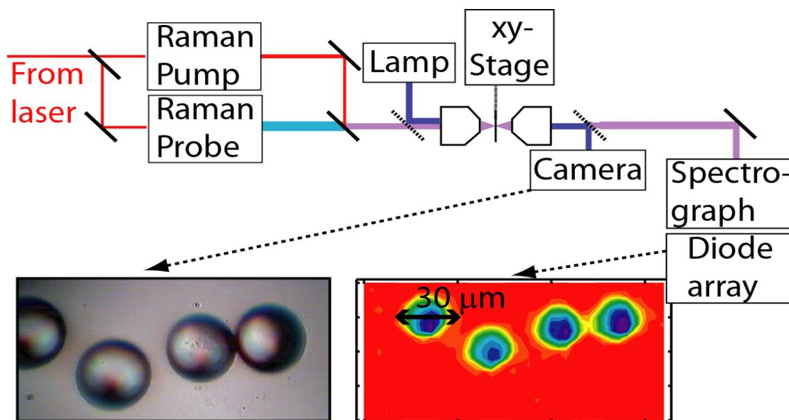
**Fig. 1:** Schematic of the FSRM set-up. The picture on the left shows a conventional micrograph of polystyrene beads dispersed in water. The false color image on the right is based on a two-dimensional array of Raman spectra. Spectral integrals covering the C-H stretch region are indicative for the polystyrene concentration and are contour-plotted here.
