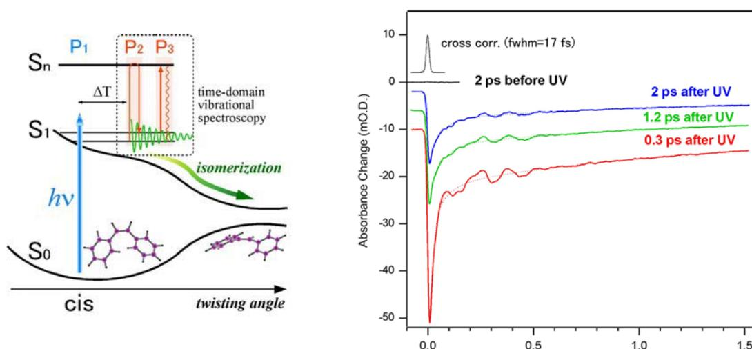
Fig.1 Scheme of TR-ISRS measurement (left) and the data of *cis*-stilbene in hexadecane (right).
