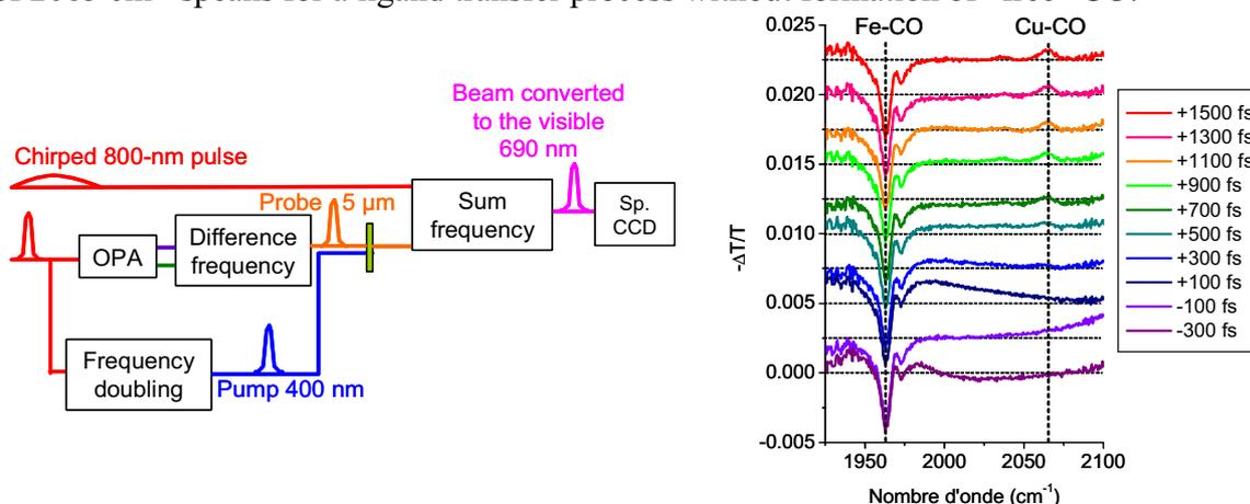
Left: Scheme of the experimental setup (Sp.: spectrometer). Right: Differential transmission spectra for pump-probe delays between -300 and +1500 fs. The spectra have been displaced vertically for clarity.
